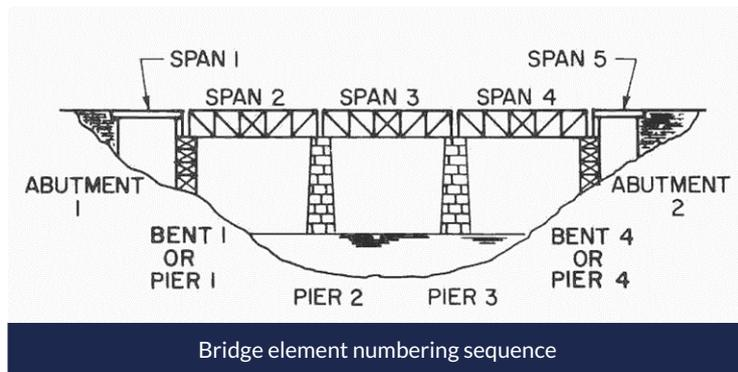
The superstructure element numbering system should include the spans, the main beams, the secondary elements (diaphragms, transoms, etc) and, in the case of a truss, the panel points. The spans should be numbered consecutively, with Span 1 located at the beginning of the bridge. Multiple beams should be numbered consecutively from left to right facing in the route direction (refer Figure 2, page 9).
