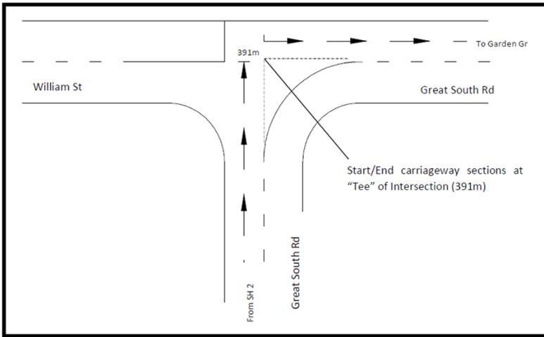
**Carriageway Section Definitions for a Through Road Making a Right Angle Turn in an Intersection**
